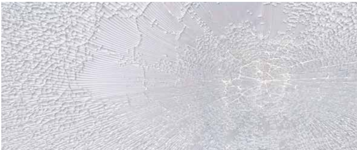
StoVentec Glass panels remain intact with little or no spalling after impact and blast.
